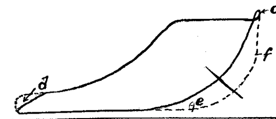
Fig. 283. Valve With Too Much Lead.
